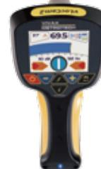
The vLocCam2 Sonde and Camera locator is a lightweight, durable locator with a full color display. The vLocCam2 Receiver comes standard with sonde/camera frequencies of 8kHz, 33kHz, 512Hz, 640Hz, power and radio. Push button depth displays the depth of cover.
