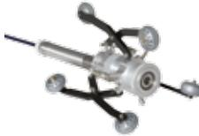
The Type "B" Adjustable Skid, for the D46/SL, is used for larger diameter pipes in lines from 8 to 15 inches in diameter. The Type "B" Skid is made of aluminum with stainless steel hardware and polyurethane wheels.
